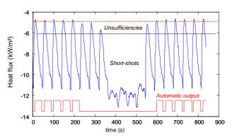
Heat flux signal during continuous injection cycles. Each peak is associated to the heat transferred during one shot. The red signal corresponds to the output of electronic device attached to the sensor.
