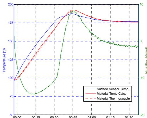
Heat Flux, Measured and Computed Composite Temperature (in red) seen from outside of vacuum bag.
