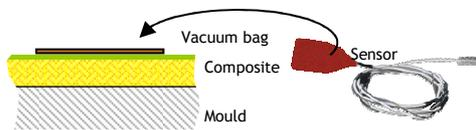
Non intrusive sensors do not disturb the processing cycle since they do not touch the part.
